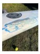
Oops, forgot to take a photo of the original damage, but this photo shows the amount of sanding required to remove the damaged gel coat and expose the sodden materials underneath.
