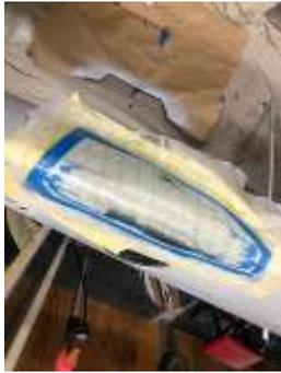
Three layers of fiberglass layed-up with epoxy resin and peel ply to take out excess resin and any trapped air.
