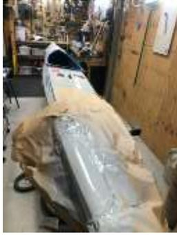
4-5 layers of grey gel coat, then the blue pin stripe will be taped up, sanded and painted with 3-4 coats.
