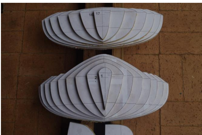
The forms around which the strips were glued show the cross-section of the hull.
