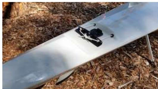
Vajda provides a small, black plastic rudder with their Club/Basic (glass) construction, which is clearly fit for purpose. However, I took the distributor's advice and upgraded to a carbon rudder in a larger size, which is beautifully made and stunning to look at. The larger rudder definitely aids in stability and has an added benefit of helping to wash-ride (or so I am told).
